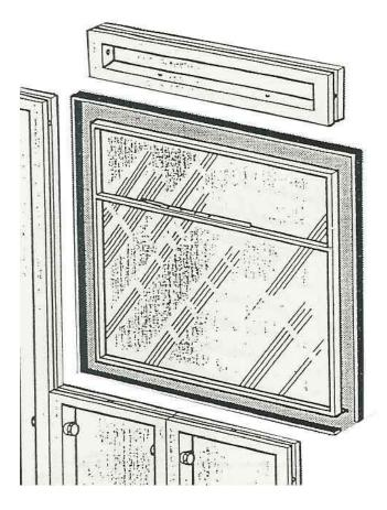
Where required, a window consists of the frame, two short panels and a lintel. Butt the short panels together and to a standing standard panel. Secure with **bolts** 4" (100mm) long, nuts and **tapered washers**.
