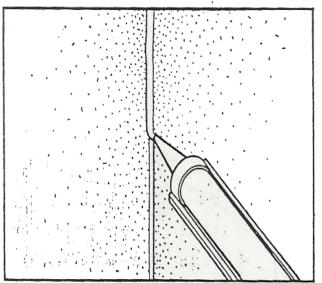
Silicone all internal joints with clear silicone as detailed above.
